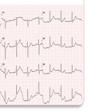
Mortara's Best 10 algorithm evaluates ECG noise to determine the best quality 10 seconds of data recorded by the ELI<sup>™</sup> electrocardiograph. So, no matter when you press the ECG button, you get the best quality ECG for review even if your patient moved in the last 10 seconds.
